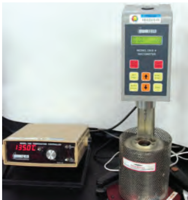
Fig. 3. Brookfield rotary viscometer according to PN-EN 13302
