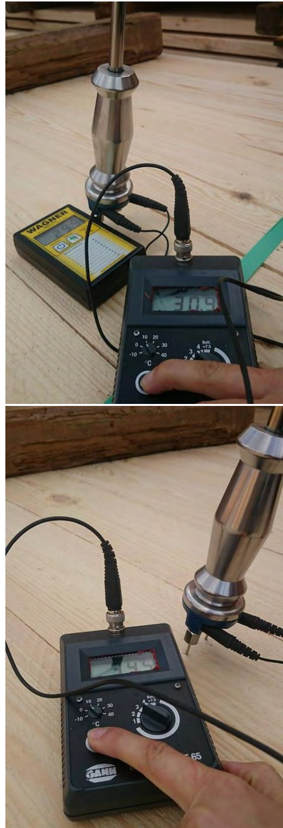
Fig. 1. Measuring the moisture content of the fresh sortment using the HT 65 GANN moisture meter [6-7]
