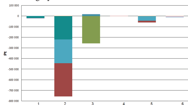
Fig. 4. The second air report: damage function modeling in 6 impact assessment categories calculated by IWM-PL software: 1 – carcinogens, 2 – organic compounds in the human respiratory system (HRS), 3 – climate changes, 4 – inorganic compounds in the HRS, 5 – acidification, 6 – ecotoxicity
