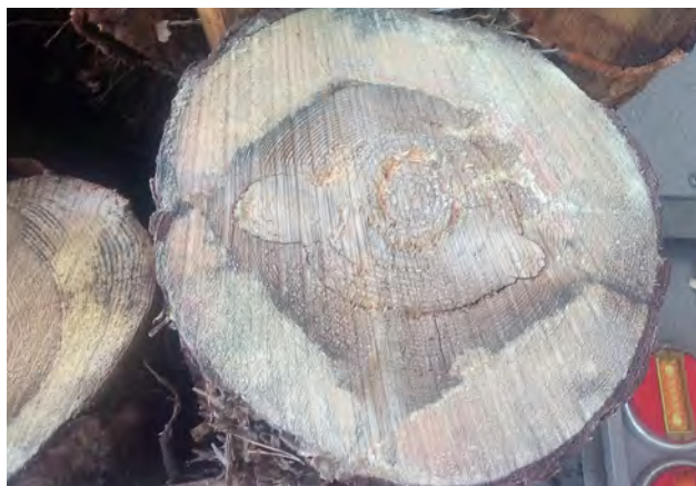
Fig. 3. Example of whorl knot arrangement in round wood of pine ( Pinus sylvestris L)
