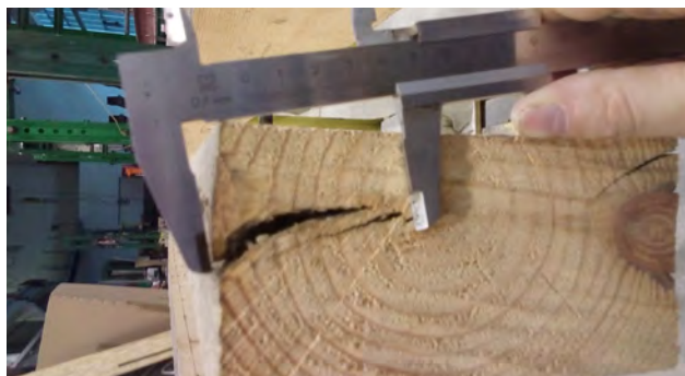
Fig. 5. Separate crack measurements in construction and structural sawn timber
