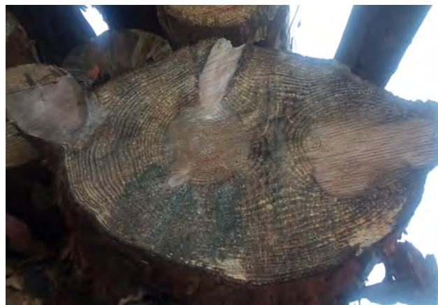
Fig. 3. Example of whorl knot arrangement in round wood of pine ( Pinus sylvestris L)
