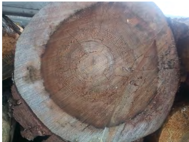
Fig. 4. Pith cracks in pine wood
