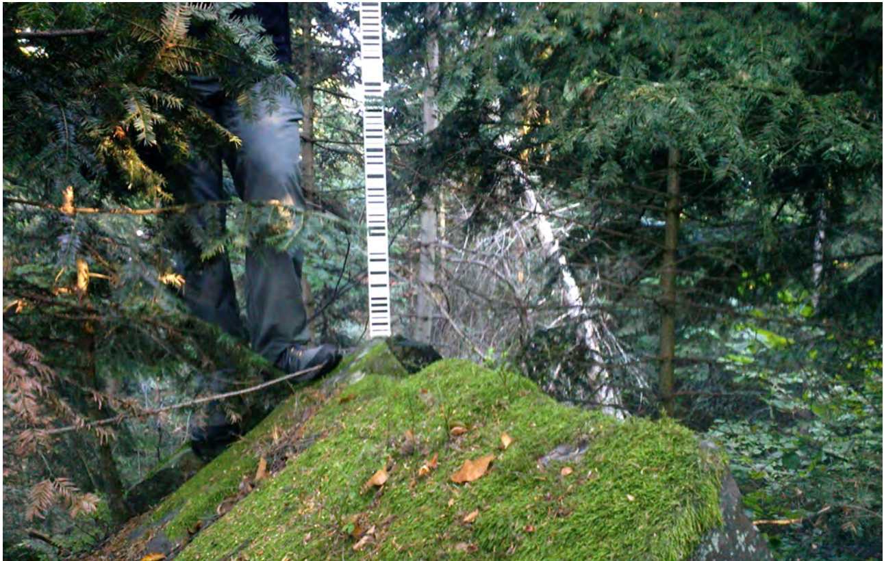
Fig. 3. Spot height survey on the top of Skala Agaty rock – differential leveling
